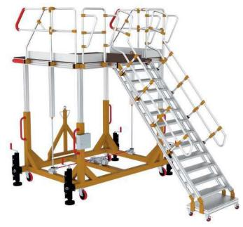
The Cargo Door Access Stand is designed for access to the AFT Cargo Door and FWD sections of the aircraft. It can be manufactured as height adjustable or fixed. Elevation options are available with screw jack, electric motor or hydraulic assembly.
