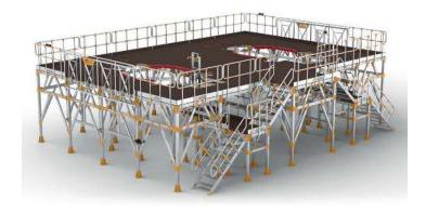
With the Airbus Sa Section-19 Shell & Barrel Platform, Section 19 part of Airbus Single Corridor (A319/320/321) aircraft is produced and these Barrels are combined with Section 18 panels and sent to Airbus Hamburg FAL facilities.
