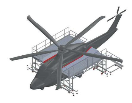
Helicopter Maintenance Stands are compatible with many helicopter models. Special stabilizers are used for height adjustment depending on whether the fuel tank is full or empty. Further height adjustment can be achieved with mechanisms such as screw jacks or electric motors.
